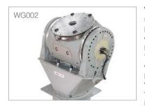
Wedge options can be special-ordered for applications in which the configuration requires the positioner to be pre-tilted. Applications include downward tilt of Roll/EL positioners in which the wedge's resulting tilt shifts the elevation travel beyond its normal downward-look
