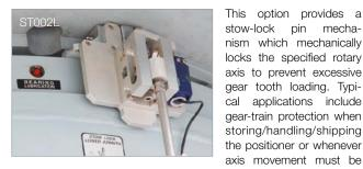
avoided (ex: when mounting a vehicle). Stow-locks operate in one of two positions: stowed in housing or installed in the axis. When the stow-lock pin is removed from its housing and installed on the positioner, a special circuit breaker (normally closed – N.C.) causes an electrical shutdown to prevent operation. Stow-locks are typically installed at 0° position. Special positions are available. Consult your local sales representative when configuring this option.
