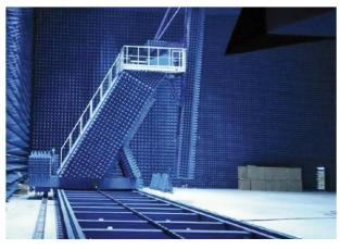
Heavy duty floor slide with inclined positioner
