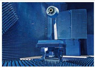
Model tower positioning system in compact range
