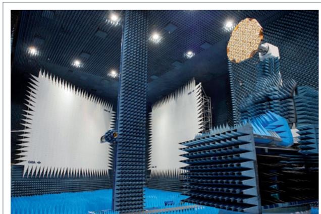
**Figure 1** - Compact Payload Test Range (CPTR) at ESA-ESTEC\* (Noordwijk, The Netherlands). A Compact Range and a NF System share the same measurement environment. Echoes and stray signals may occur while performing NF measurements.
